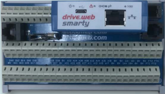
dw240-DM-C3CD only 5.51" wide x 3.43" high x 3.0" deep (140mm x 87mm x 76mm)
