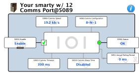
**Comms Timeout**. The time in millisecond, ms, for the master or client to wait for a reply before moving to the next parameter in the polling cycle.
